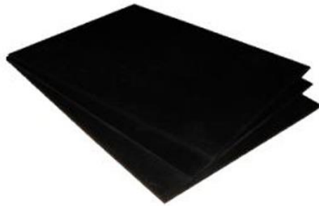
Figure 8 – Image of Resonant Rubber-Based Microwave Absorber Source: Soliani EMC (2021).
